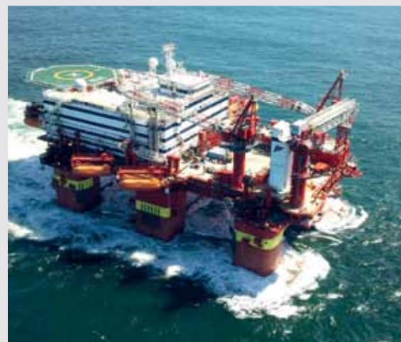
Floatel Superior is the first DSS™ 20NS accommodation semi built for the North Sea
